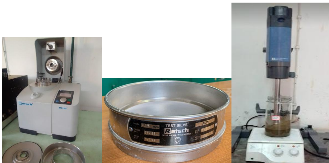
Figure 12: Mill, 200 mesh sieve and ultraturax rotator
