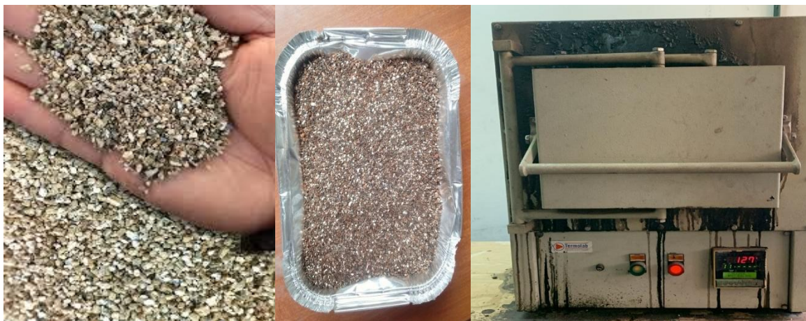
Figure 11: Raw vermiculite and high temperature muffle furnace
