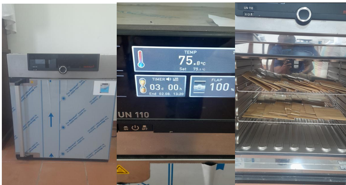
Figure S1.12. The Memmert 30-1060 UN110 Universal Oven used for drying samples at 75 °C for 3 days to achieve constant weight.
