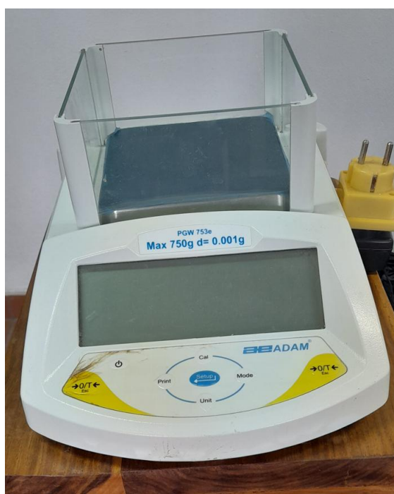
Figure S1.13. The Adam Precision Balance (accuracy \pm 0.001 g), used for weighing samples.
