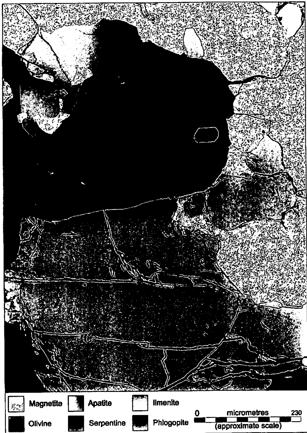
Figure 5.10 Head sample, false coloured backscatter image.
