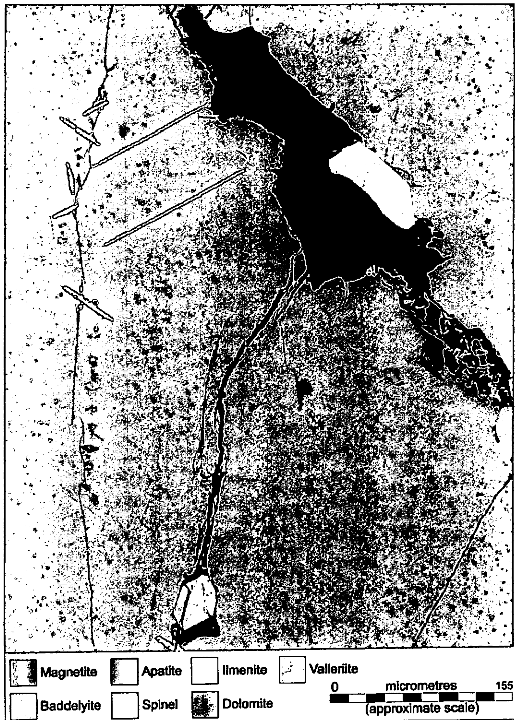
Figure 5.8 Head sample, false coloured backscatter image
