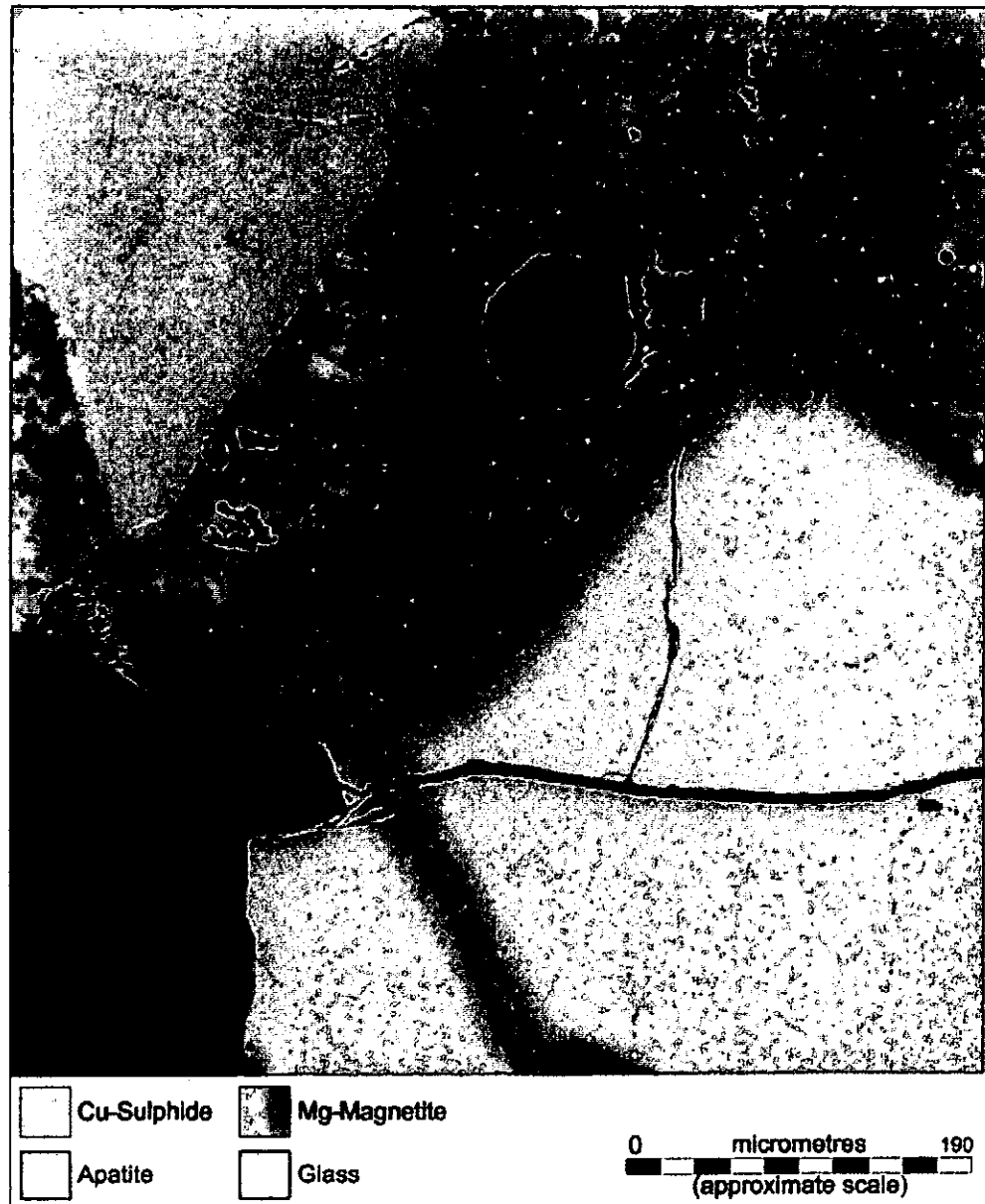
Figure 5.20. 240 Second treated sample, false colour backscattered image (after Kingman 1999).
