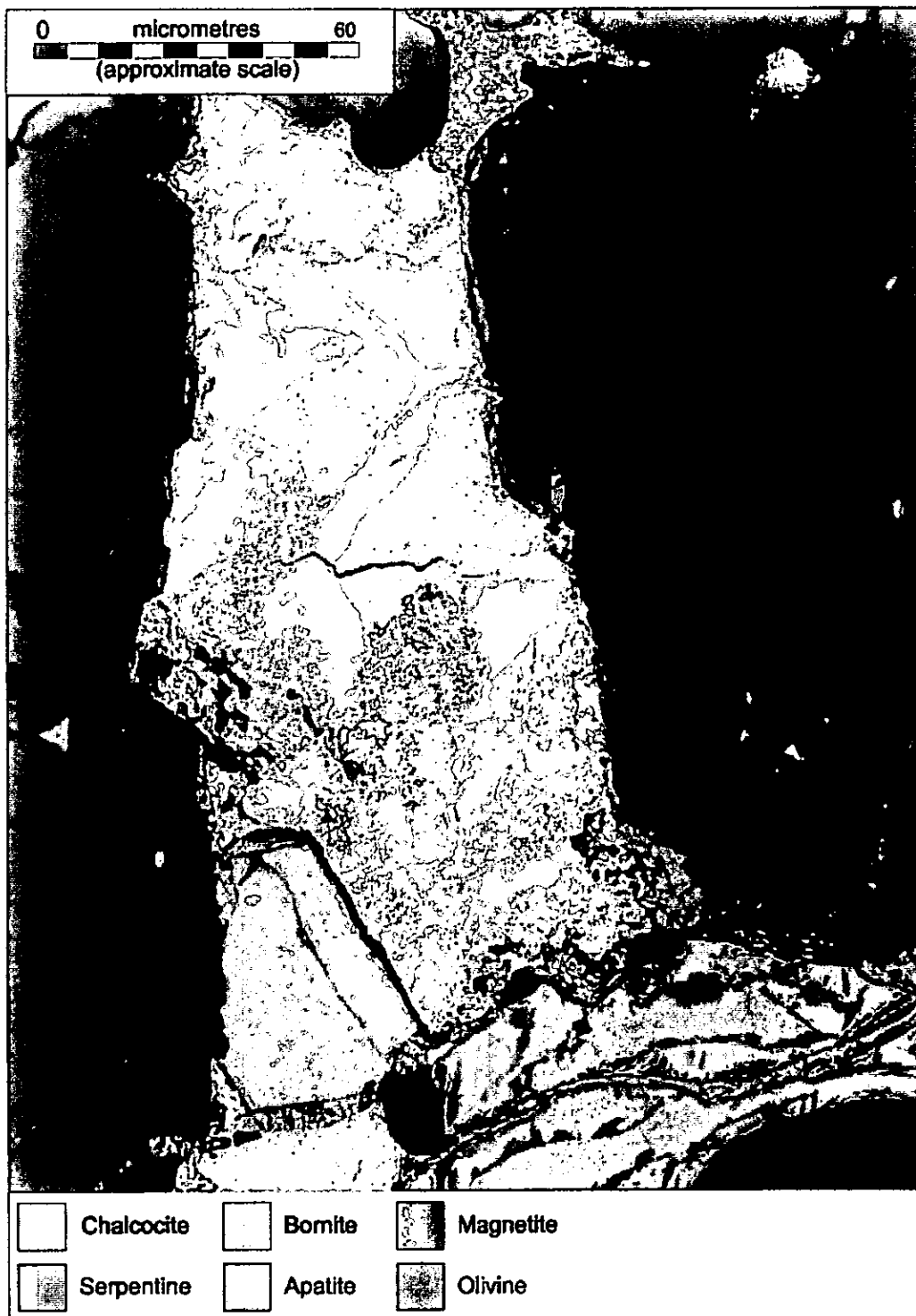
Figure 5.12 Head sample, false coloured backscatter image.
