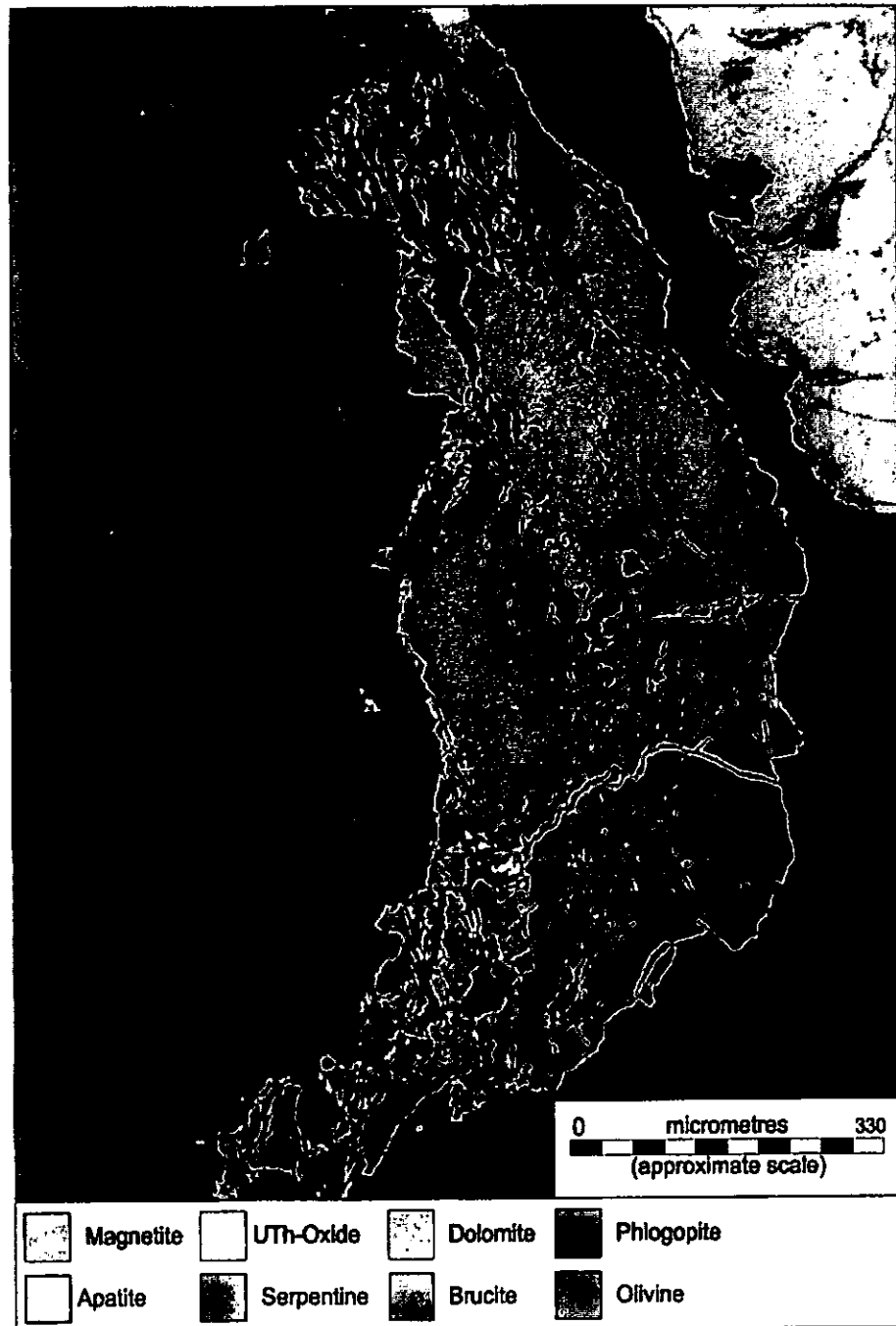
Figure 5.9 Head sample, false coloured backscatter image
