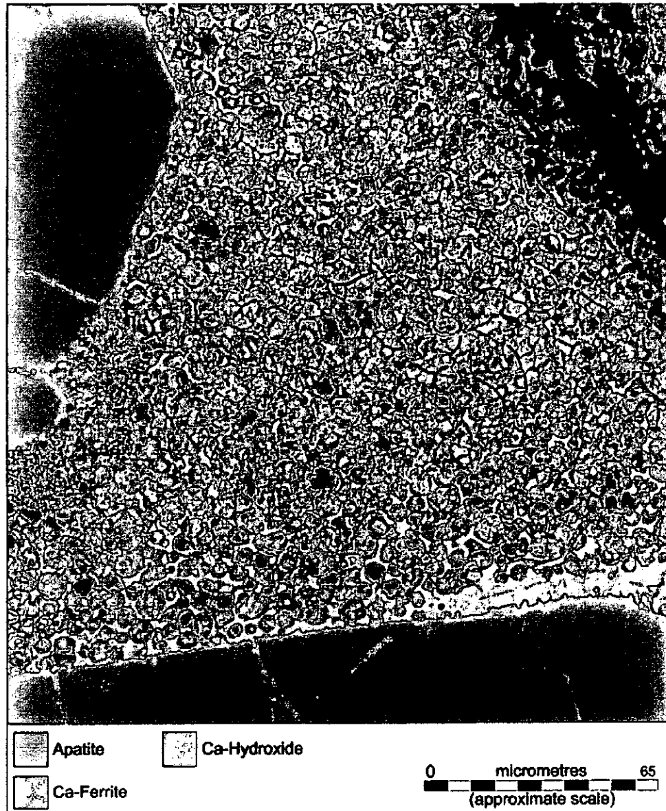
Figure 5.21. 240 Second treated sample, false colour backscattered image (after Kingman, 1999).
