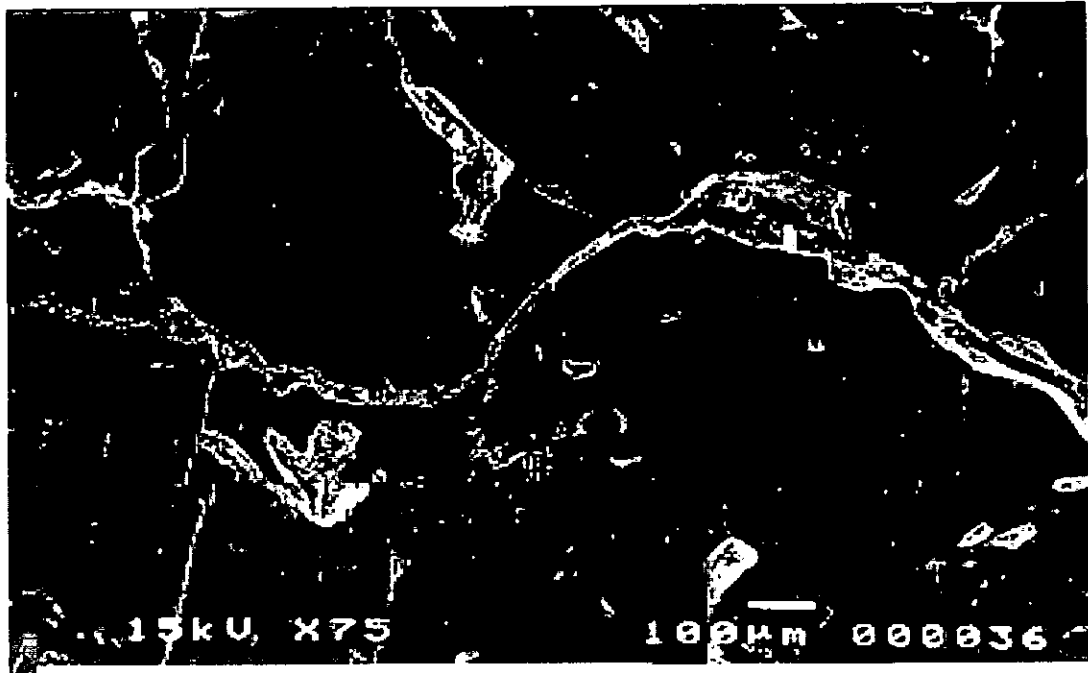
Figure 3.2 Typical Intergranular microwave Induced Fracture on a Norwegian Ilmenite (after Kingman et al., 1998)
