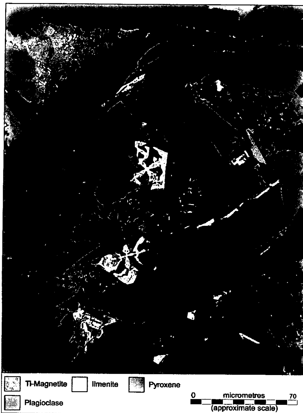
Figure 5.15 Head sample, false coloured backscatter image
