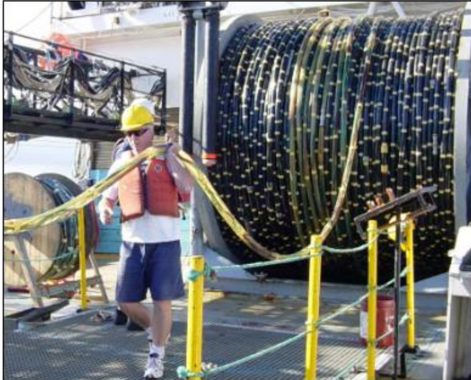
Figure 2. 7: A streamer being deployed into the water. When the vessel is not acquiring seismic, the streamer is kept onboard coiled on a reel. (Alfaro et al., 2007; Telford et al., 1989).
